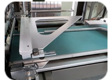
“APA” Automatic Product Size Adjustment of Inverting Triangle & Infeed Conveyor *Exclusive Feature!
