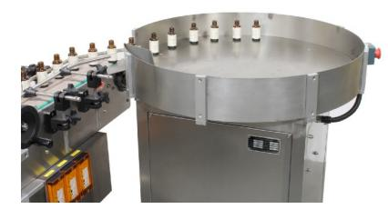
Level transition plate fits next to existing conveyor to facilitate easy transition from one conveyor to another.
