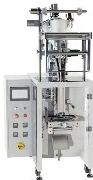
(Top) G-300F equipped with auger filler for powders
